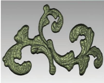
**8** The next step is working on the exterior of the perfume bottle, where I'll bring the surfaces for the scroll work, heart and body into the CAD system (in this case Pro/E Wildfire) and stitch all the components into a solid model.
