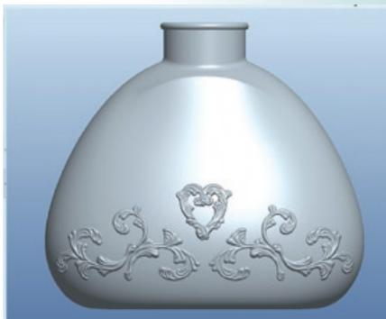
**9** The final step is creating the internal shell. These surfaces are now so complex that most CAD systems could not generate them accurately, but voxel modelling in Geomagic Freeform lets me easily create the shell volume:
