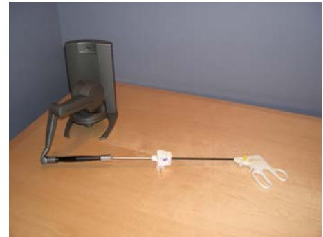
The PHANTOM Desktop haptic device with the Auto Suture ® 5mm Endo Clinch ® II device attached.
