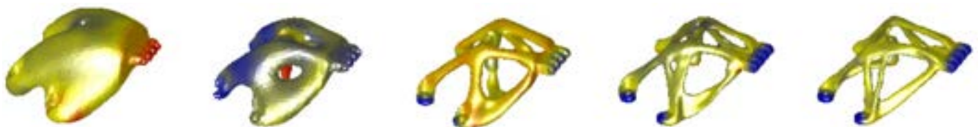
The evolution of a part, from the first iteration to the optimized lightweighted version.
